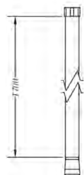
Ref.: 100140 30 Flexo 1,70 m. PVC antirrotura y tuerca loca PVC flexible hose 1,70 m anti-breaking and swiveling nut
